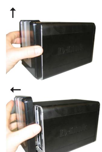
3. Insert a 3.5" SATA hard drive into each available drive bay. Make sure to align the drive connectors to the SATA connectors on the bottom edge inside the drive bay of the DNS-323. Gently push the drive in until it connects. When a drive is inserted properly, you will feel it "seat" into the connector. Some hard drives that are thin or oddly shaped may need to be guided carefully into position. If a drive is not properly seated, the light will not illuminate after powering on the device.
